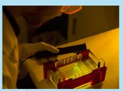
FastGene<sup>®</sup> BG-LED Flashlight: Originally developed for the detection of fluorescent DNA dyes.
