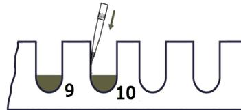
[ 5 ] Press
