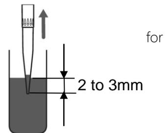
When replacing the tip, pre-rinse the tip with the necessary dispensing volume setting. The reverse operation is recommended for a sample liquid that tends to linger in the tip.
