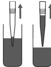
[ 2 ] Put the tip end into the receiving vessel and press the
