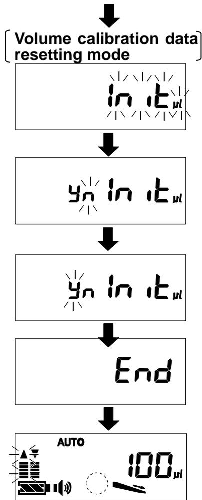
[ 3 ] Press the Up or Down key to select volume calibration data resetting mode.
