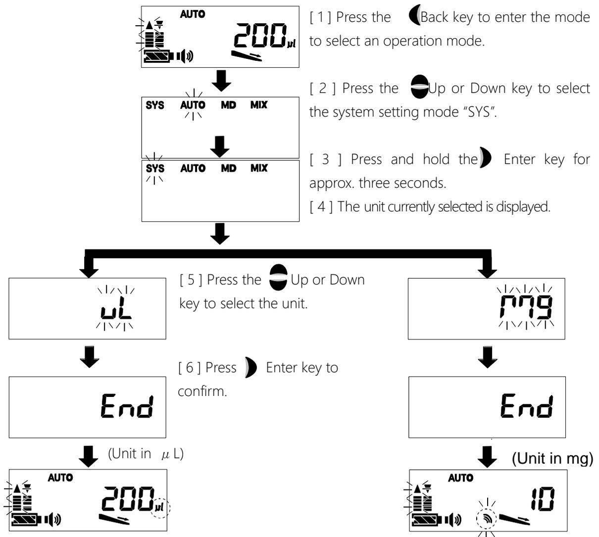
With the  $\mu$  L unit selected, the Notice mark is turned off while the  $\mu$  L unit mark lights up.
