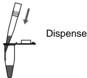
[ 3 ] Press the
