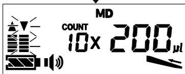
[ 2 ] Put the tip end into a receiving vessel and press the
