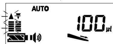
[ 1 ] Put the tip end into the liquid to be dispensed and press the
