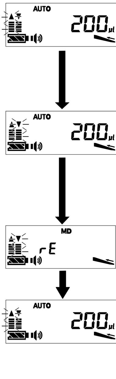
[ 1 ] Press the
