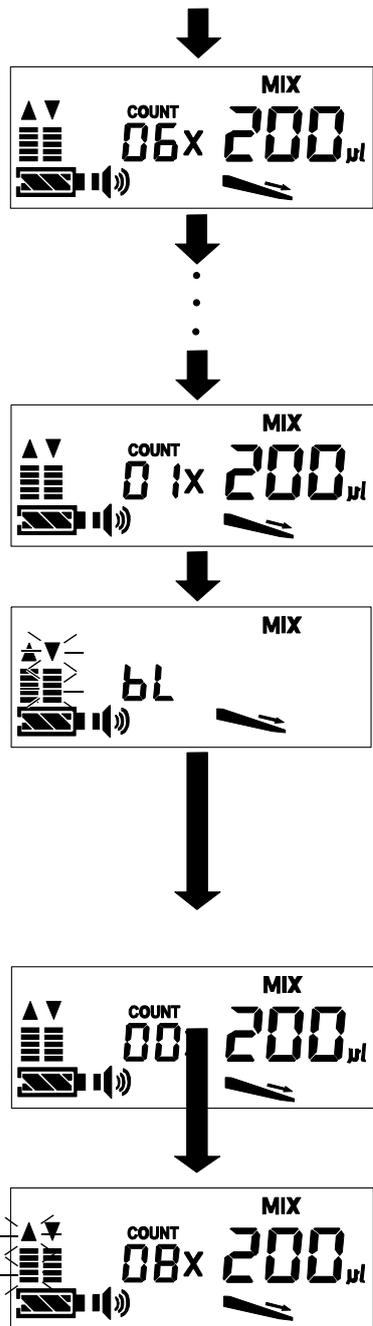
[ 3 ] The pipette executes the set count of aspirating-dispensing cycles by approx. 2/3 of the set mixing volume.
