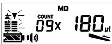
[ 3 ] In a similar manner, put the tip end into the next vessel and press the
