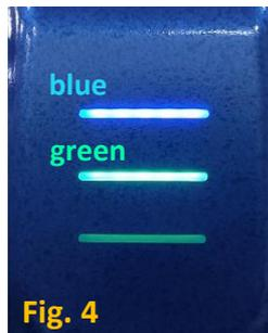
\*The green flashing LED shows the instrument is successfully ready for connection. If not, please repeat the step 4.
