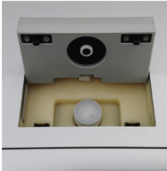
Figure 3-7 Push the cartridge to the bottom
