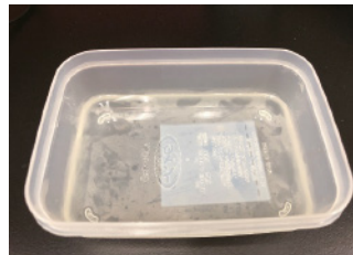
TAE buffer with MGX in same concentration as in agarose gel (MGX 4 \mu L/TAE 100 mL)
